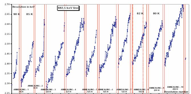
Plot of SPI’s energy resolution of the 882.5 keV line as a function of time, showing the effect of the bi-annual annealings.
