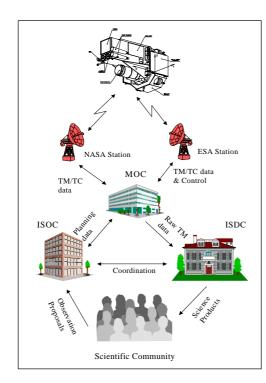
The INTEGRAL Ground Segment (see figure) consists of the Operational Ground Segment (OGS) and the Science Ground Segment (SGS).
