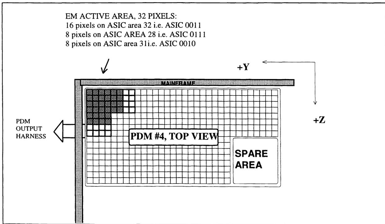
Fig. 5 Schematic of the module EM detectors position
