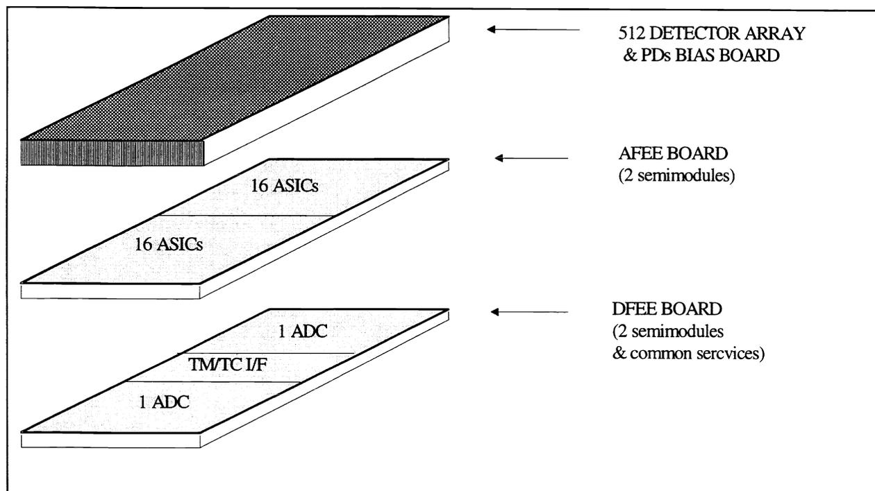
Fig. 2 PICsIT module assembly
