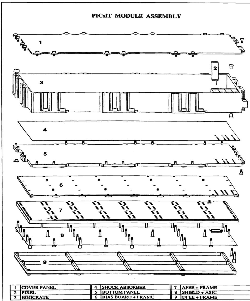
Fig. 4 Exploded view of the module structure.
