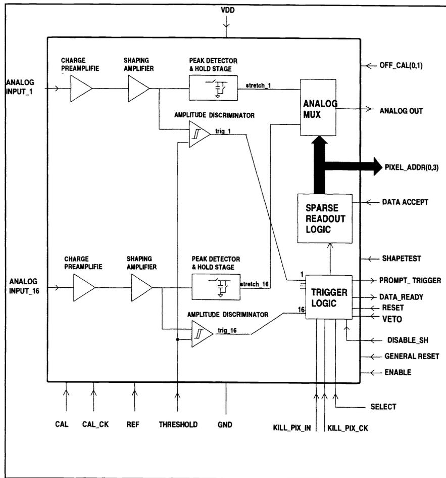
Fig. 3 ASIC schematic diagram
