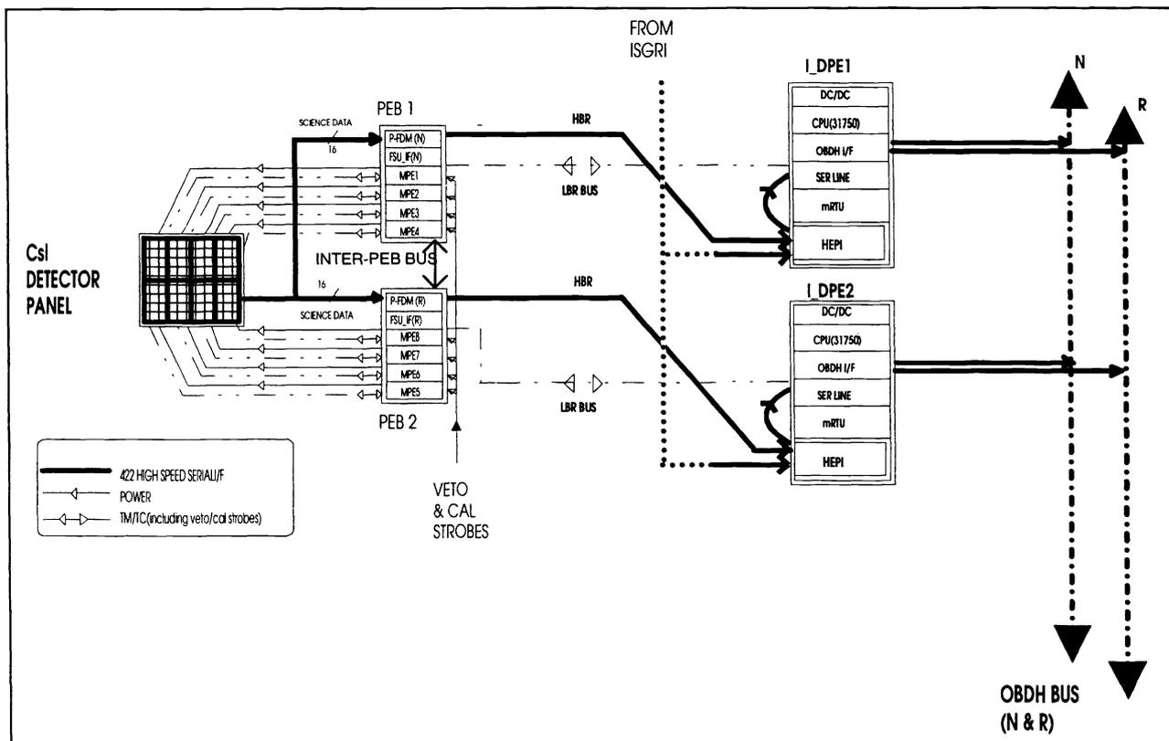
Fig. 1 PICsIT block diagram
