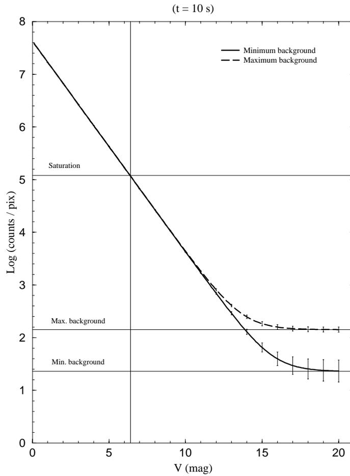
Figure 8: Expected number of counts on the central brightest pixel as a function of V magnitude, for an integration time of 10 s. The error bars correspond to  $1\sigma$ . The plot also includes the expected background flux computed for maximum and minimum conditions.
