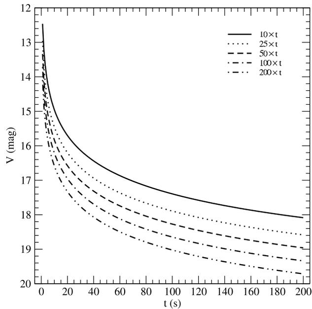
*Figure 7: Limiting faint magnitude for a  $3\sigma$  detection in the V band as a function of integration time. Best case background conditions are assumed (galactic pole, no zodiacal light). The curves correspond to different total numbers of images being combined.*
