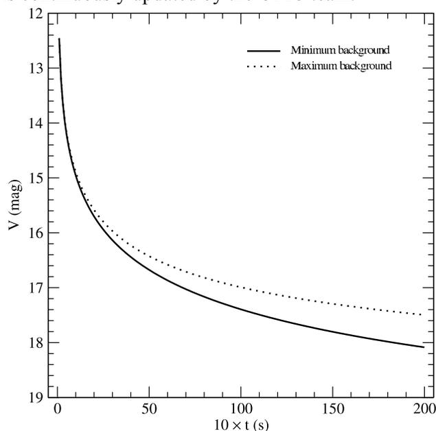
Figure 6: Limiting faint magnitude for a  $3\sigma$  detection in the V band as a function of integration time. The best and the worst background cases are shown. It is assumed that 10 separate exposures, each with the integration time as given in the plot, have been combined together in order to increase the signal to noise ratio.
