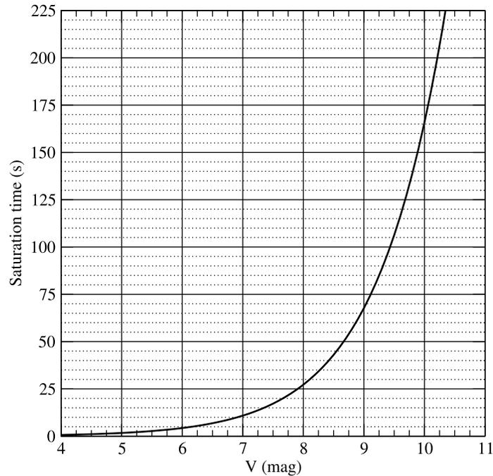
*Figure 9: CCD saturation time as a function of V magnitude. Note that for integrations of 50 s, all stars with  $m_V < 8.6$  will saturate the CCD. For the shortest OMC integration times (fast monitoring mode: 3 seconds), the brightest stars that can be observed should be fainter than  $m_V > 5$ .*
