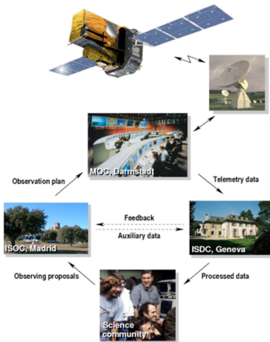
Figure 4: The INTEGRAL flight and ground segments.
