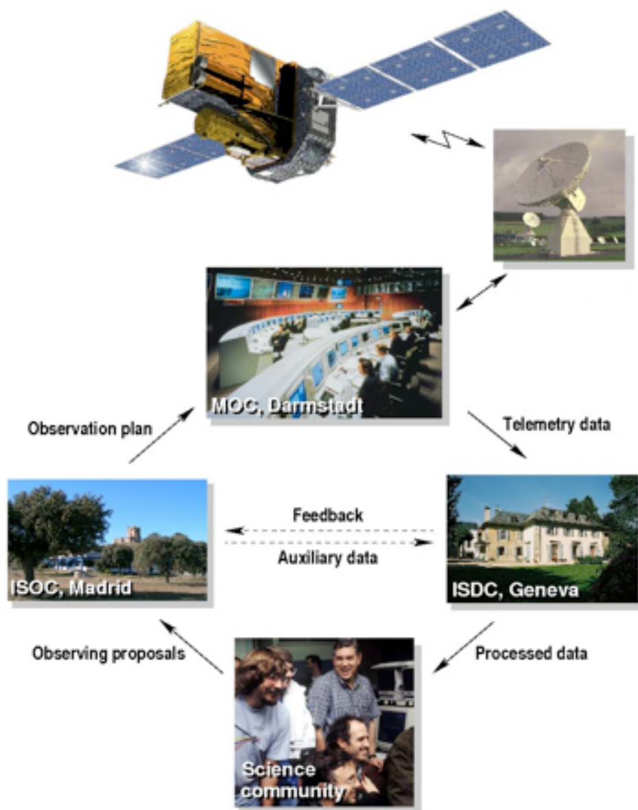
Figure 4: The INTEGRAL flight and ground segments.
