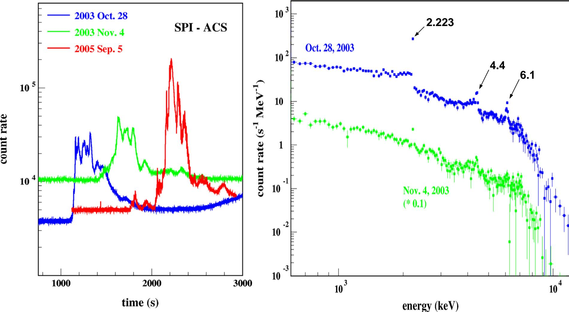
lines: 2.223 MeV [ ${}^1\text{H}(n,\gamma)$ ], 4.4 MeV ( ${}^{12}\text{C}$ ), 6.1 MeV ( ${}^{16}\text{O}$ )
