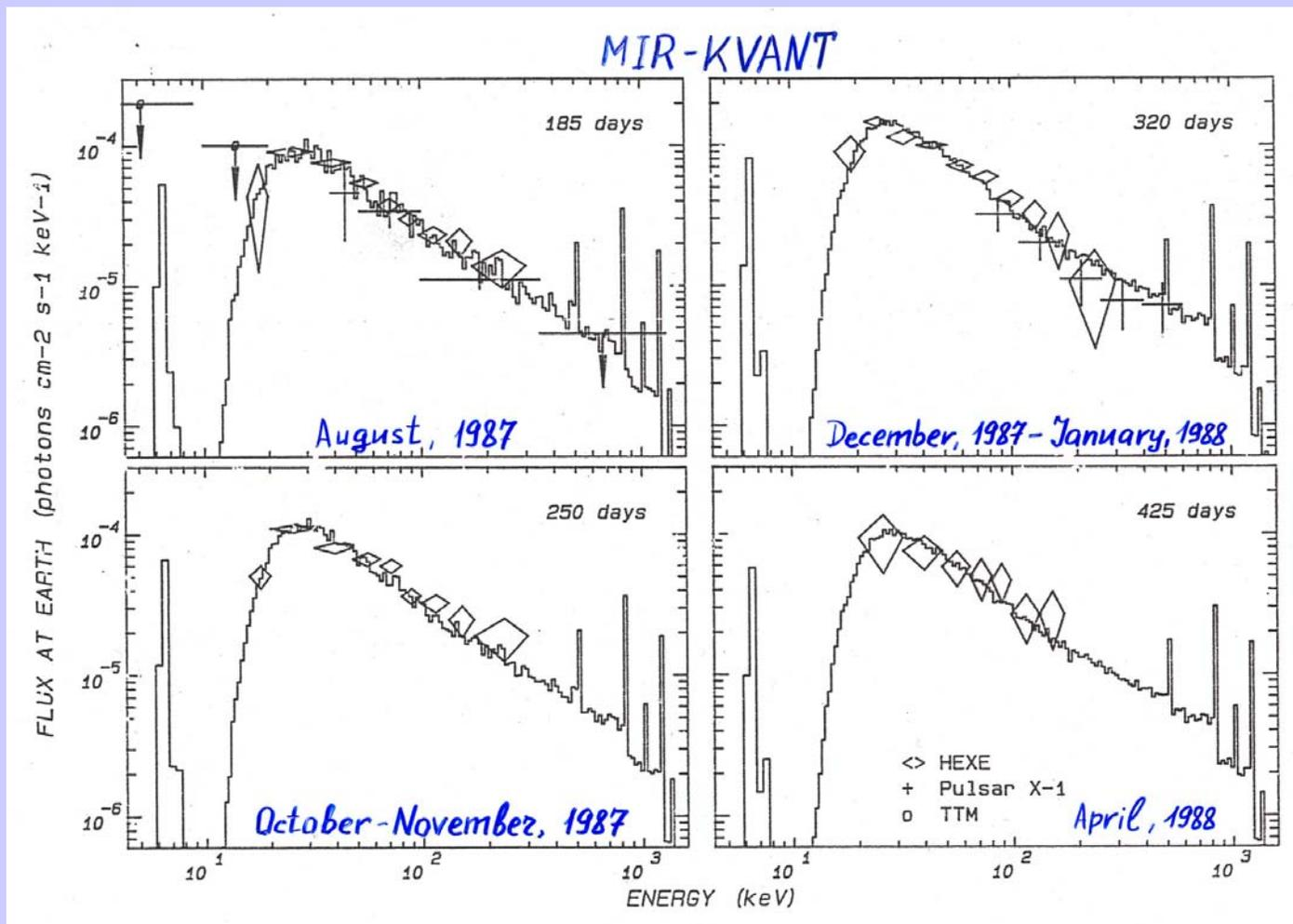
*Evolution of the hard X-ray spectrum of SN1987A as measured by MIR-KVANT and its explanation by radioactive decay of  $^{56}\text{Co}$  and Comptonization.*
