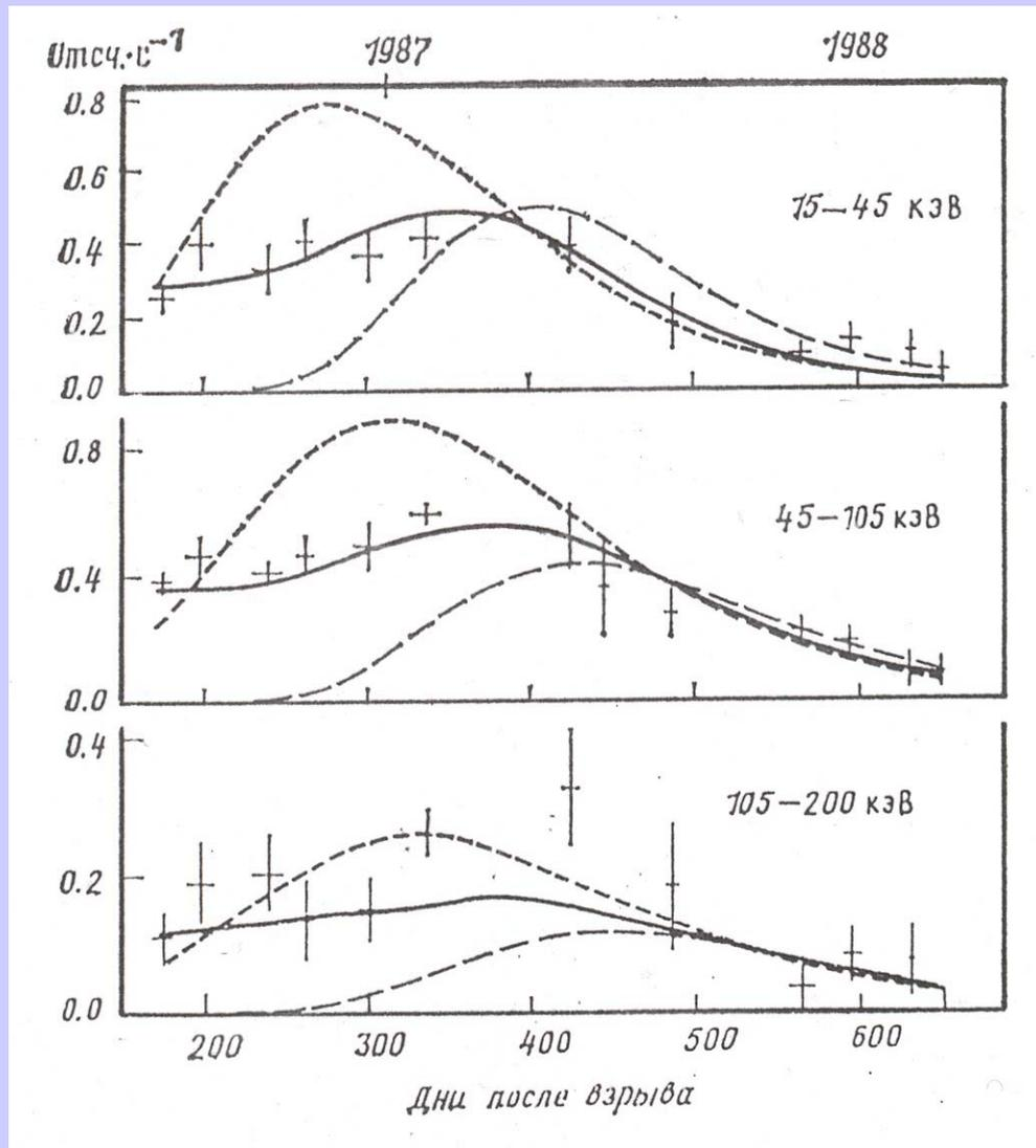
Evolution of X-ray flux from SN1987A as measured at different energies with HEXE and its sensitivity to  $^{56}\text{Co}$  mixing.
